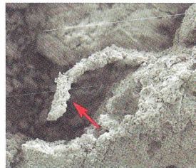
UltraFiber 500 achieves excellent bonding with cement
