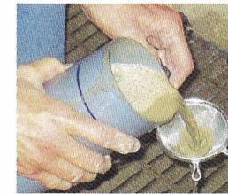
Screen wash pre-set concrete with a sieve
